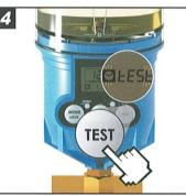
Turn on the lubricator and press the TEST button for 2 seconds to run a test cycle. The unit will start to dispense oil and operate continuously in purge / test mode. This process will last approximately 2 minutes to ensure every function of lubricator works properly.
